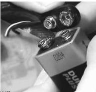
4. Carefully, in order not to damage the wire, disconnect the old battery.
