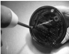
2. Remove the screws from the lid and open the call bell's case.
